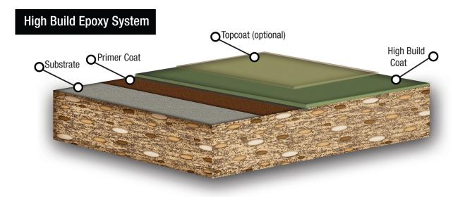
High Build Epoxy System is a high build, colored epoxy/urethane, high performance concrete coating system. It is used for environments requiring an attractive, high performance floor or when a concrete floor has sustained damage requiring a moderately thick surfacer.
